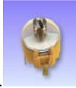
adjust the capacitor's capacitance.
