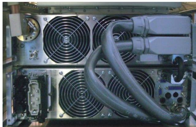
Figure 5-1 Example of PJ5000U-K installation in a rack
