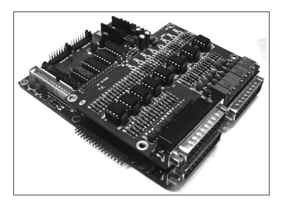
The telemetry card also makes the contacts of eight relay switches available in output (max. 24V - 0.5A).
