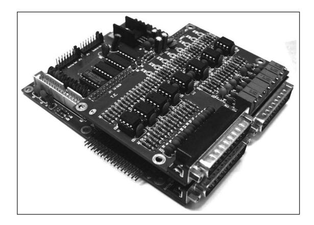
The telemetry card also makes the contacts of eight relay switches available in output (max. 24V - 0.5A).
