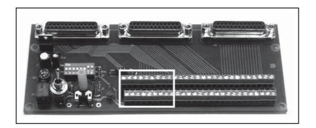
Inside the white rectangle are evidences the clips relative to the 8 balanced analogic inputs described in the following table.
