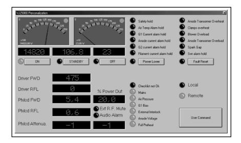
In order to change some levels such as attenuation of the inputs and the output power percentage of the PTXLCD, double click on the measurement that you wish to change and insert the new value required.
