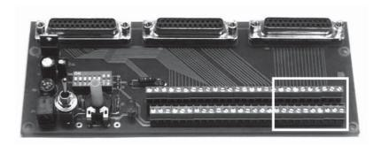
Inside the white rectangle is evidences the clips relative to the 8 relay outputs described in table.
