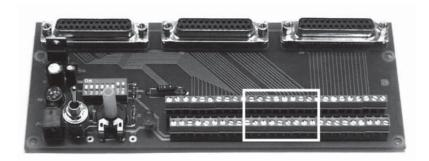
Inside the white rectangle is evidences the clips relative to the 16 Digital/Analogic inputs described in table.
