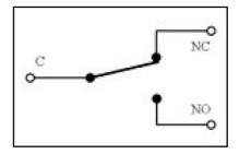
The maximum current that could be made flow through the contacts is of 500mA to 24V.
